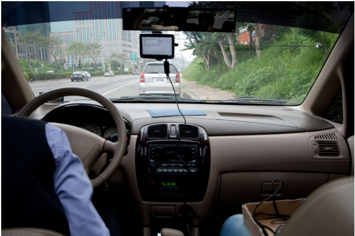
Fig3-1. TMC2001 installation with PND.
