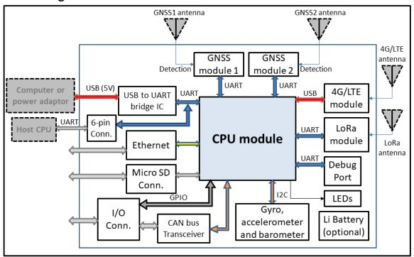
The blocks with the dashed outline are not included in the product. GNSS module 2 is only included in RTK-M101 and RTK-M101R. LoRa module is only included in RTK-M100R and RTK-M101R.
