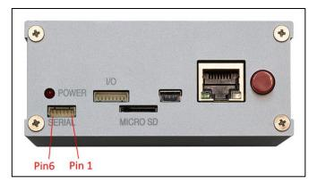
TX and RX signals of the serial port and USB-UART bridge IC connect to the same UART port of the product's internal CPU module. If both serial port and Mini USB connector are connected, the serial port will dominate the communication with the internal CPU module.
