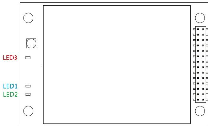
Blue LED flash (location on **LED1**, 1Hz): Means the receiver is normal operation
