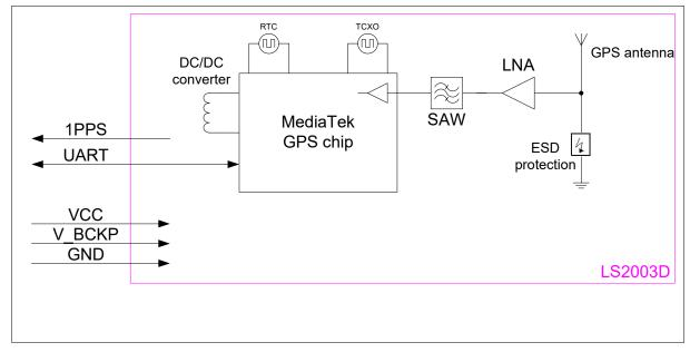
Fig 3-1 System block diagram of LS2003D
