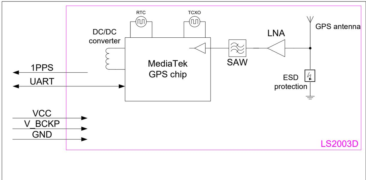
Fig 3-1 System block diagram of LS2003D
