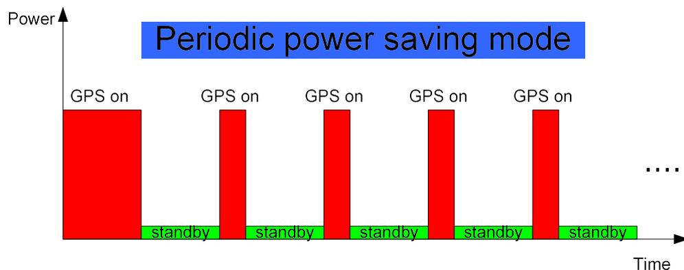
The following flow chart is an example to make GPS module go into periodic mode and then back to normal operation mode.
