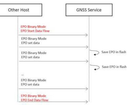
Figure 9. The sequence of the EPO flash aiding
